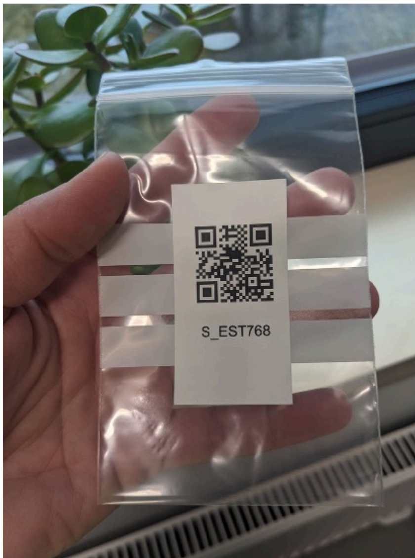
Figure 6. QR code sticker on a sample bag, ready for scanning with the PlutoF GO app. Photo credit: Inga Hiiesalu-Vahter.
